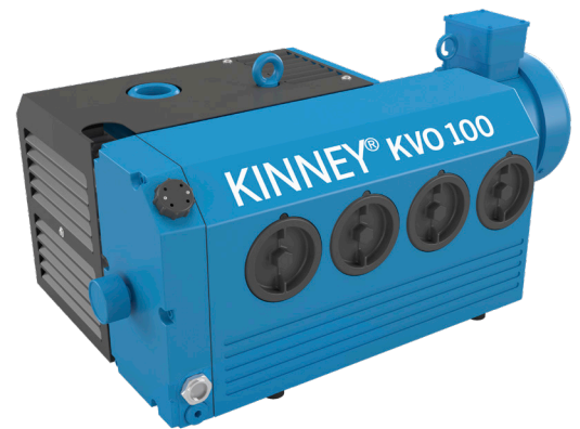
KVO100 exterior oil separator elements.
