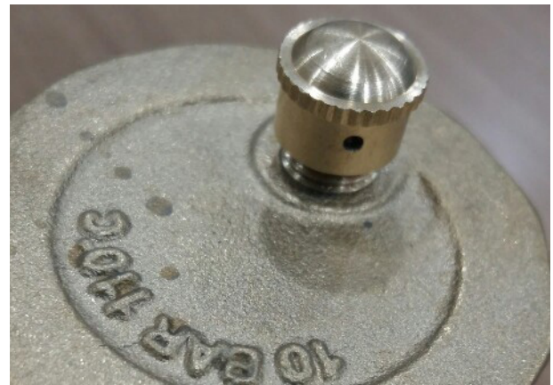
Figure 4-1 – SDV air vent cap.
